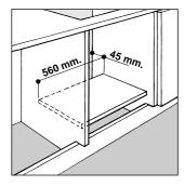
To fasten the oven to the cabinet, open the door of the oven and fasten it by inserting the 4 wood screws into the 4 holes locate on the perimeter of the frame.
